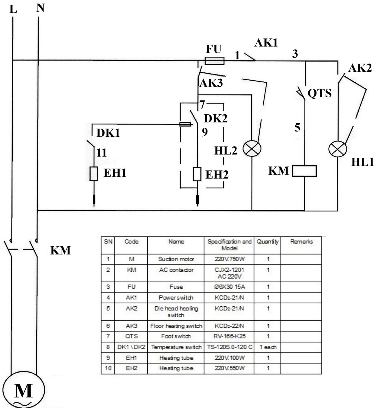
Figure 4 : Electrical Schematic Diagram of KW-303 Ironing Table
